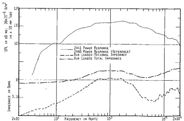
Fig. 15. Power response and air-loaded impedance of a 2441 compression driver.
