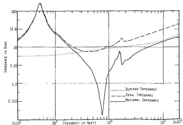
Fig. 6. Motional impedance in vacuum of a 2420 compression driver.
