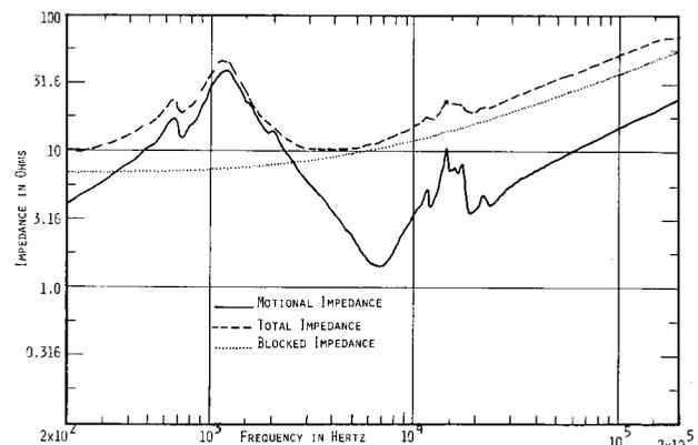
Fig. 14. Motional impedance in vacuum of a 2441 compression driver.
