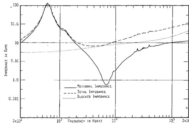
Fig. 8. Motional impedance in vacuum of a rejected 2420 compression driver.
