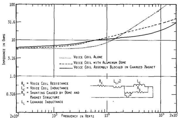
Fig. 4. Blocked voice-coil impedance.
