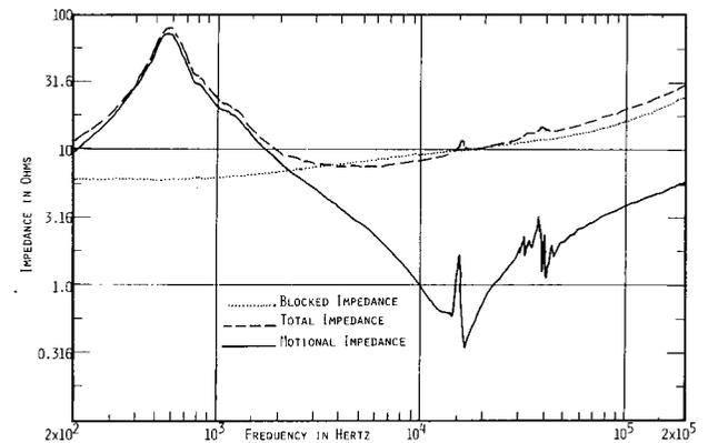
Fig. 10. Motional Impedance in vacuum of a 2421 compression driver.
