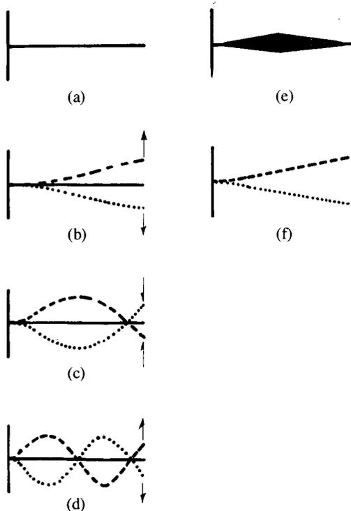
Fig. 2. Vibrational modes of a beam. (a) Clamped-free uniform beam. (b) First eigentone  $f_1$ . (c) Antinode  $f_2 = 6.27f_1$ . (d) Second eigentone  $f_3 = 17.6f_1$ . (e) Nonuniform beam. (f) First eigentone.
