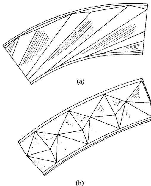
Fig. 3. Three-dimensional suspension concepts. (a) Tangential surround. (b) Diamond-shaped surround.
