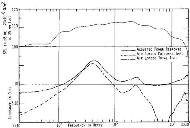
Fig. 7. Power response and air-loaded impedance of a 2420 compression driver.
