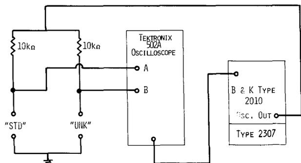
Fig. 5. Block diagram of motional impedance bridge.
