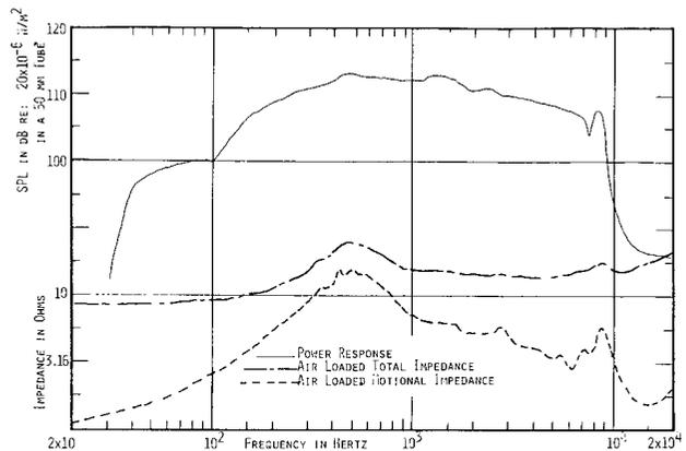
Fig. 13. Power response and air-loaded impedance of a 2440 compression driver.
