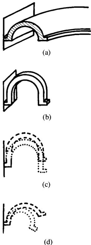
Fig. 1. Half-roll suspension. (a) Solid annular half-roll. (b) Sliced roll with legs. (c) Linear motion of sliced roll. (d) Complex motion of solid half-roll.
