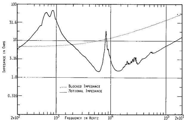
Fig. 12. Motional impedance in vacuum of a 2440 compression driver.
