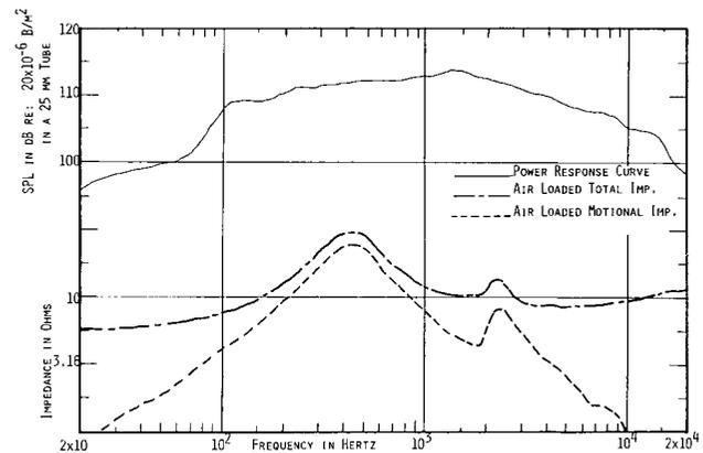
Fig. 11. Power response and air-loaded impedance of a 2421 compression driver.
