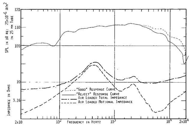
Fig. 9. Power response and air-loaded impedance of a rejected 2420 compression driver.
