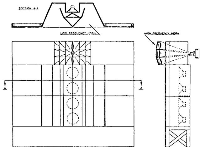
Fig. 4. Shearer two-way horn system, folded type.
