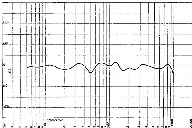
Fig. 3. Output characteristic of Shearer horn system measured on normal axis and 10 ft (3 m) from horn.
